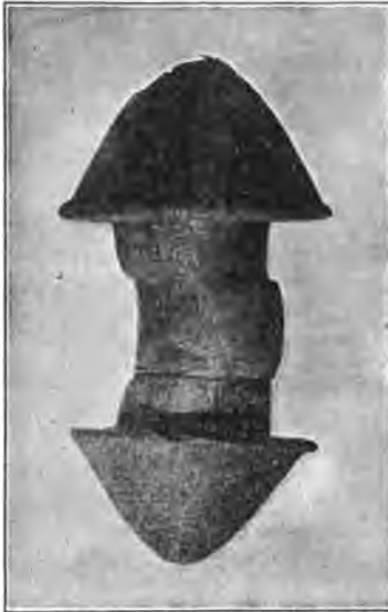
Fig. 51. — Failure of Rivet.
